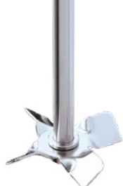
figure 2: This 4-blades mixer is one tool used for miscible liquid-liquid mixing.
