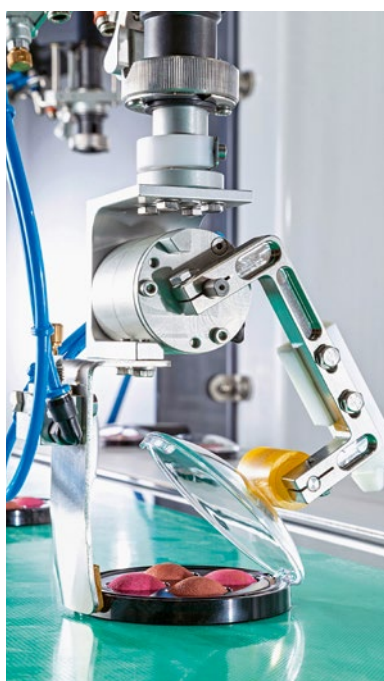
Once all the colour palettes have been glued in place, an F4 robot equipped with a specially developed tool closes the box
