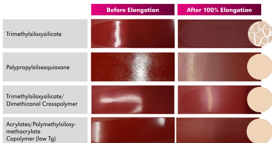
fig. 3: Silicone resins and silicone resin gums film flexibility
