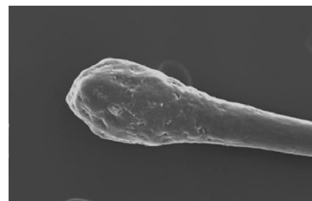
fig 4: SEM imaging of the hair tip following 2% lipopeptide treatment, slow-drying and straightening
