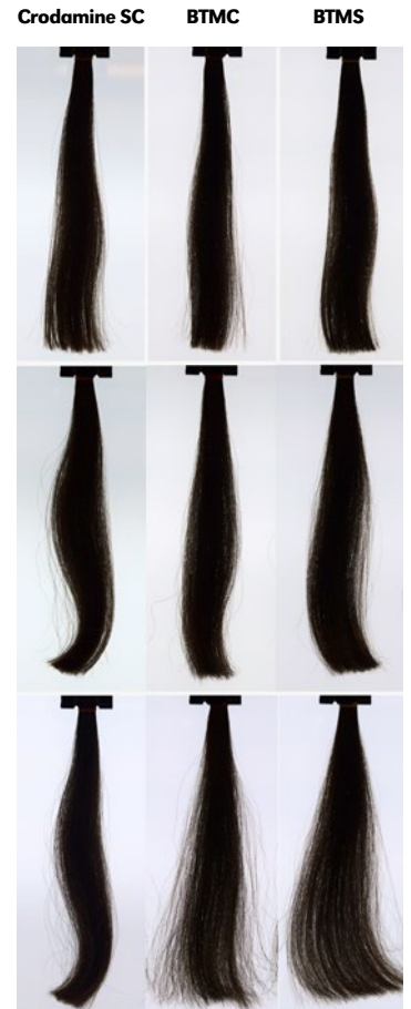
fig. 1: Untreated hair tresses, after treatment with either Crodamine SC, BTMC or BTMS and after treatment and combing ten times
