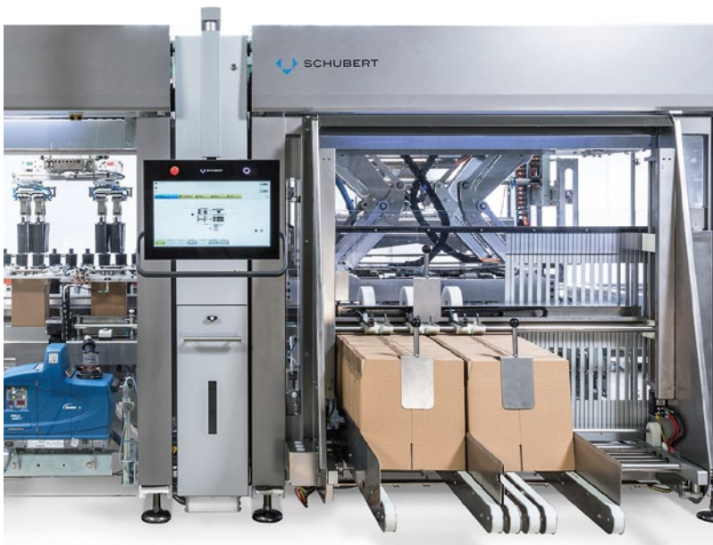
Schubert-Cosmetics Fully automated adjusted to a wide range of format sizes: RSC carton magazine and erecting tool.
